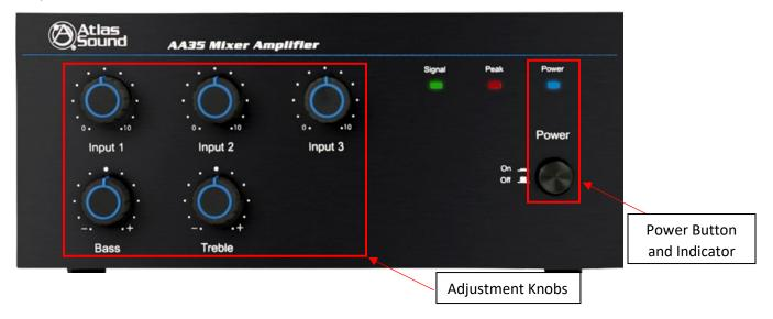
*Power Button:* Used to power on/off the amplifier. Power on is indicated by a solid blue light on the Power indicator and power off is indicated by no light on the Power indicator.
